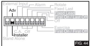
The Alarm / C.A. DIP switch selects whether a combustion air damper or alarm device is to be connected to the C.A. / Alarm terminals (12 and 13) (FIG. 45).
